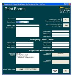
Enter the battery expiry date (marked on the original right hand label) and the Vessel name, if known. If the users contact details are also known, please enter these in the appropriate boxes. Click on <Print> to print the programming certificate on your default printer.
