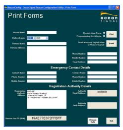
Enter the battery expiry date (etched on the top of the PLB). If the users contact details are also known, please enter these in the appropriate boxes. Click on <Print> to print the programming certificate on your default printer.
