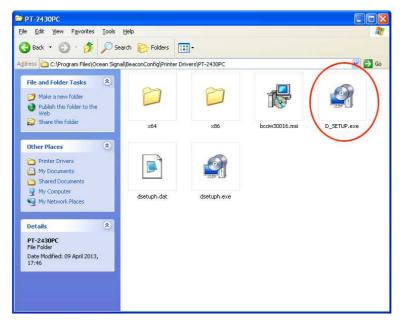
Open the folder called PT-2430PC and run the file 'D-SETUP.exe' The following warning screen will be displayed.
