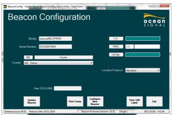
Press either the CS, MMSI or Call Sign buttons. If CS is selected the serial number will be automatically entered. (Note: It is recommended that the Call Sign option is not used and the transmitted position accuracy is severely reduced)
